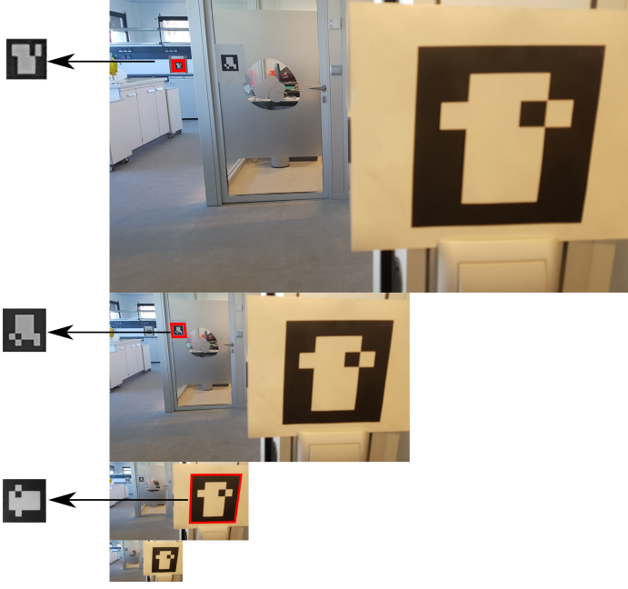
Figure 3: Pyramidal Warping. Scene showing tree marker at different resolutions. The left column shows the canonical images warped from the pyramid of images. Larger markers are warped from smaller images. For each marker, the image of the pyramid that minimizes the warping time while preserving the resolution is selected.
