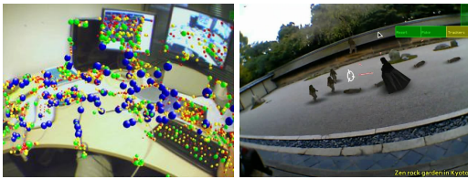
Fig. 10. Parallel Tracking and Mapping (PTAM) [57] (a video is available here )
